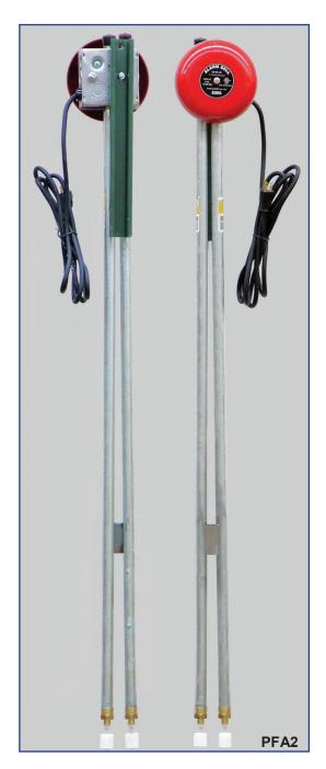
Our quality built 120VAC pit flood alarms designed for up to 4' deep pit and equipped with an 8' long power cord, 3-wire grounded plug, and 6" alarm bell. They are extremely adjustable, mounting to 8#, 12#, or 15# rails. One or two liquid level float switches installed on 4' galvanized rigid steel conduits (GRC). Mounting unistrut arm  $1-5/8" \times 13/16" \times 14"$ and hardware included.
