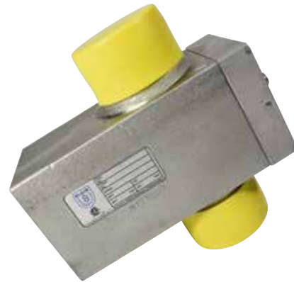
PRV-R102V Pipe Rupture Valve 2" Victaulic – Flow sensitive, pressure activated valves act as a "velocity fuse" to retard the downward motion of a descending elevator to provide gradual stop • Flow rates to 380 GPM, 50 to 640 PSI operating range • Fully adjustable closing rate, manual lowering around the valve when set • Fully adjustable flow rate minimum pressure loss in the up direction 90 degrees
