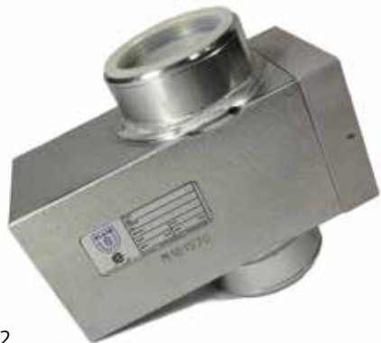
PRV-R102 Pipe Rupture Valve 2" – Flow sensitive, pressure activated valves act as a "velocity fuse" to retard the downward motion of a descending elevator to provide gradual stop • Flow rates to 380 GPM, 50 to 640 PSI operating range • Fully adjustable closing rate, manual lowering around the valve when set • Fully adjustable flow rate minimum pressure loss in the up direction 90 degrees
