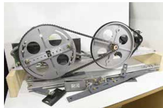
MOVFR-3N3 Door operator, center parting doors CP 40" – 49", D.O. MOVFR II, 220V, 15"
