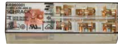
V23050-A1110-A533/SR96001 Safety Relay 6PST 3NO/3NC positively-guided 8 amp contacts w/110VDC coil Commonly used with A17 compliant controllers Equivalent to Schrack SR6A4110
