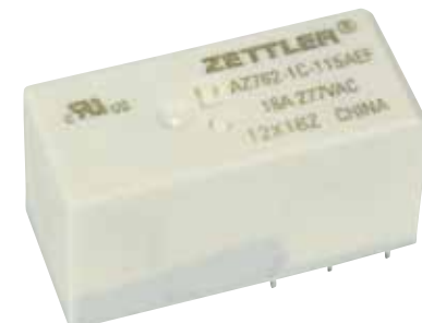
AZ762-1C-115AEF Relay 115VAC 8.1KOhm 16A SPDT
