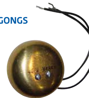
BG40W Single Stroke Must be wired in series with a 40 watt incandescent hall light
