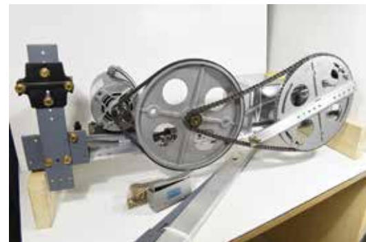
MOVFR-06R Door operator, right hand door SS-2S 45" – 48" D.O. MOVFR II, 220V, 13"
