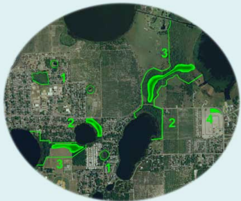
■ FIGURE 16. Strategies for permitting development in undeveloped areas of Winter Haven include (1) preserving existing low-lying, undeveloped areas, (2) enhancing and extending wetland lake fringes, (3) preserving wet corridors, and (4) requiring low-impact development. Source: Mark T. Brown for PBS&J
