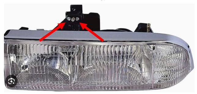
3. Also remove these screws and 10mm bolt
