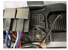
6. Next, install the bracket, and attach the upper mount, using the factory screws and 10mm nut. It should look like this:
