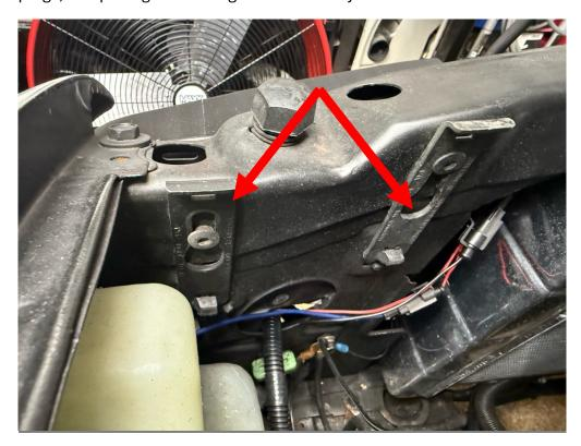
2. Remove the upper factory headlight mount, by removing the two screws on the upper mounting point.
