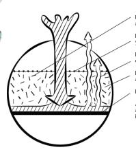
Bark fibers draw liquids to the bottom of the fill and away from the surface, leaving it dry. Netting keeps the bark fill contained, preventing
