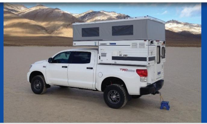
Dry Weight: 1040 Lbs. Roof/Wall Framing: Aluminum
