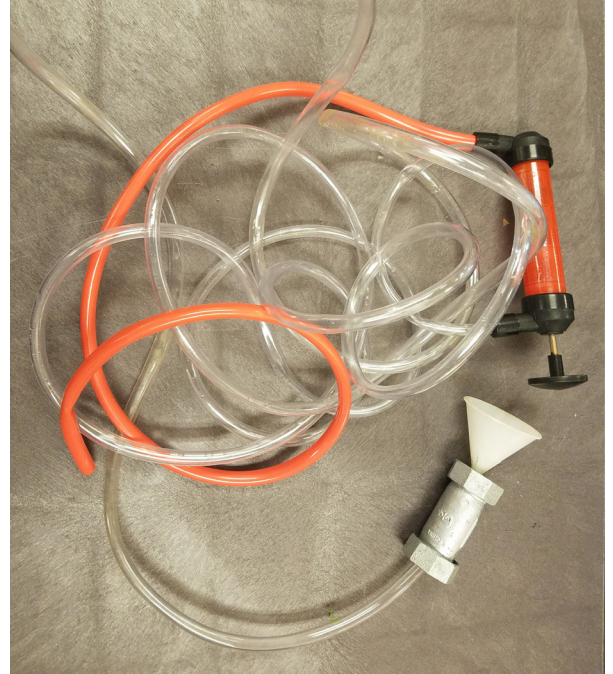
Hand pump siphon; red tube is for outflow into bucket or other container; clear tube has funnel and weight on the end for inflow
