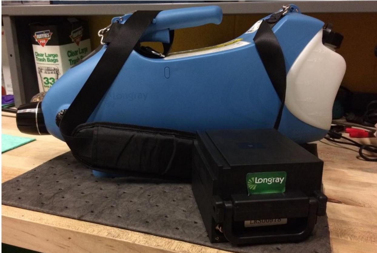
Pesticide reservoir holds approximately 64 ounces of liquid pesticide, battery lasts about an hour.
