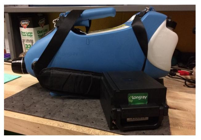
Pesticide reservoir holds approximately 64 ounces of liquid pesticide, battery lasts about an hour.
