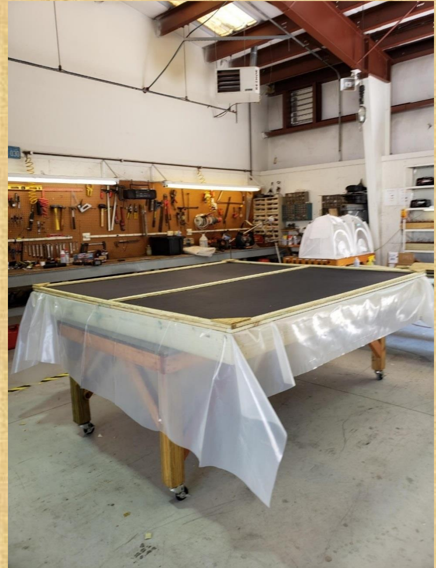
Plastic laid inside and cut to size
