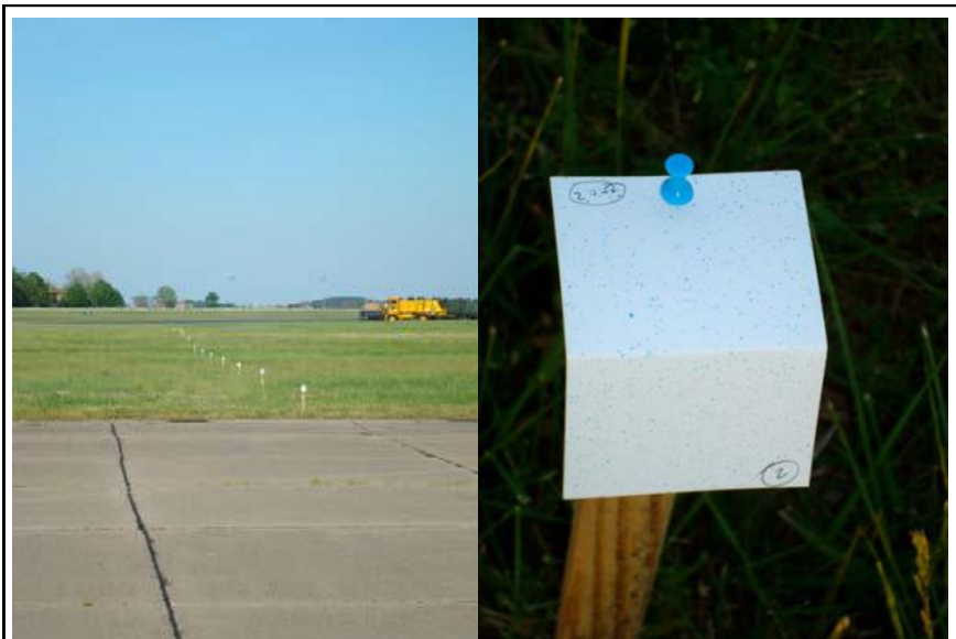
Figure 4. Spot cards used to capture dye and Bti application. Left, distribution of cards in area of application. Right, Card with dye following application.
