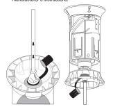
Return shroud to upright position after finishing operation. Leave tubing attached to tube-fed safety syringe and quick-fit connector until dosing equipment has been removed from the shroud. Remove dosing equipment by pushing the trigger as shown in the picture, then disconnecting the quick-fit connector from the
