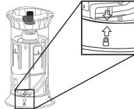
Remove the flexible cap from the fluid connection. Attach the quick-fit connector to tubing if not already attached. Push the quick-fit connector downwards onto the shroud fitting until it clicks into place.
