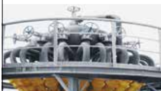
Annular Distributors AKA-SPIDER for alumina classification
