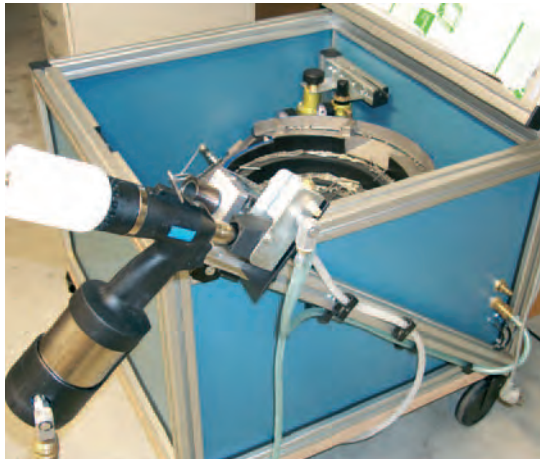
Partly automated feeding system ALFOMATIC BZ 101 A
