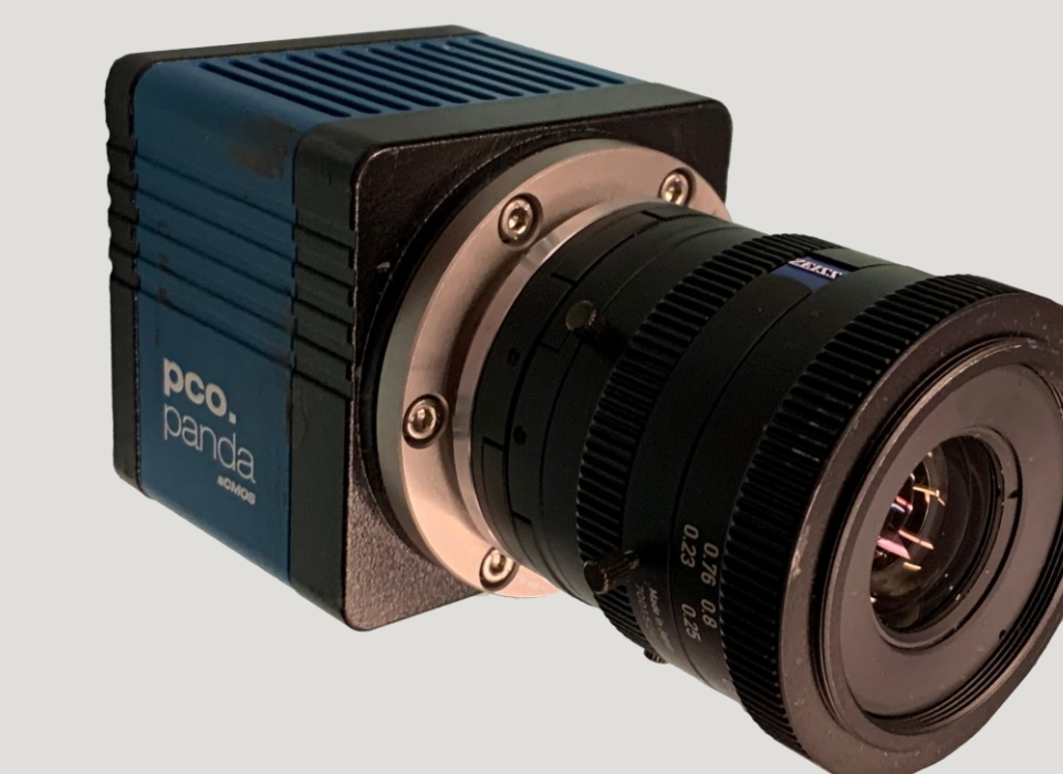
Figure 3: The Payload Flown on RSONAR 1,2 and 3
