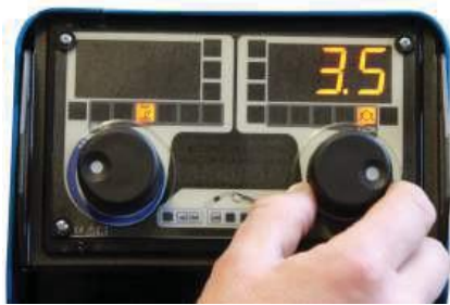
Figure 21. Feeder panel (23) Spot welding time setting Here: 3.5 sec. for MIG Synergic welding
