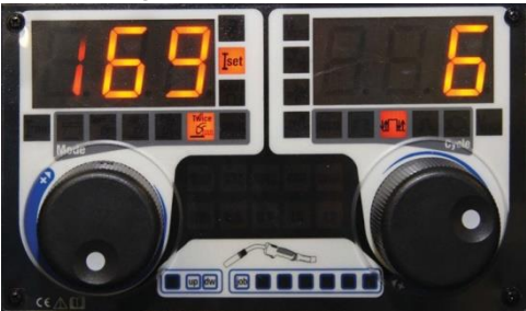
Figure 18: Feeder panel, active Double Pulse (Twice) function.
