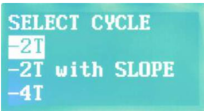
Figure 6. DPF Panel Exemplary button cycles on the welding torch. Here: 2-cycle.
