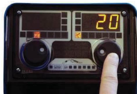
Figure 9. Feeder panel (23) regulation of inductance in MIG manual mode.
