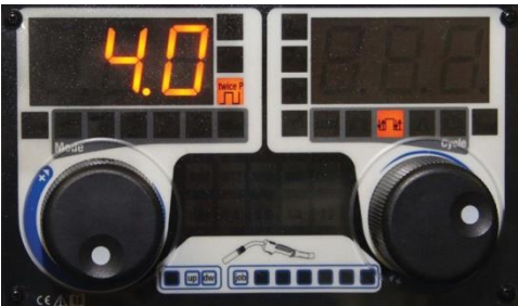
Figure 19: Feeder panel, setting of double pulse frequency. Here: 4Hz
