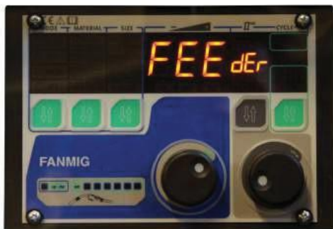
Figure 30. FEEder message on current source panel Only DPF panel is active
