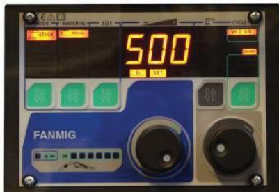
Figure 25. Current source panel, STICK coated electrode welding mode.
