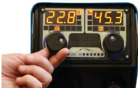
Figure 8. Feeder panel (23) Here: MIG manual, wire feed speed 22.8 m/min, arc voltage 45.3 V, 2-cycle.
