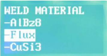
Figure 11. DPF Panel Material choice (welding programme) Here: Steel powder wire (Flux).
