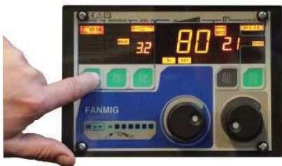
Figure 27. STICK synergic welding. Here: alkaline coated electrode of 3.2 m diameter, 80A welding current, 2.1 mm suggested material thickness, VRD function switched on.
