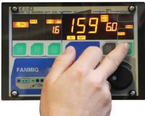
Figure 28. TIG synergic setting Here: SG2 steel 1.6 mm wolfram electrode diameter, 159 A welding current, 6,0 mm material thickness to be welded, 2-cycle with current drop.
