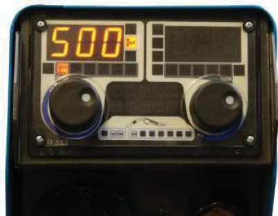
Figure 24. Feeder panel, welding current setting for MMA electrode - 500 A.
