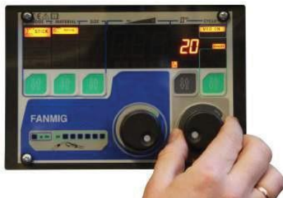
Figure 26. HotStart setting. Here: Hs 20.
