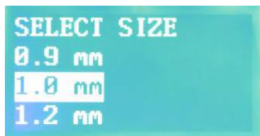
Figure 12. DPF Panel Choice of wire diameter Here: 1.0 mm
