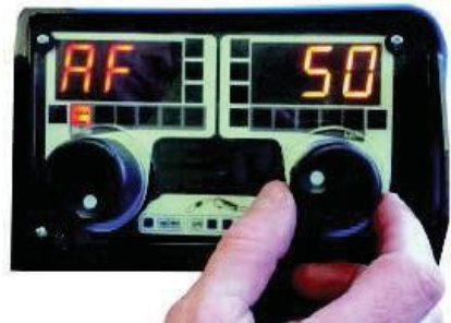
Figure 22. Feeder panel (23) ArcForce function setting Here: ArcForce 50.
