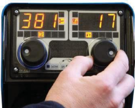
Figure 15. Setting arc length
