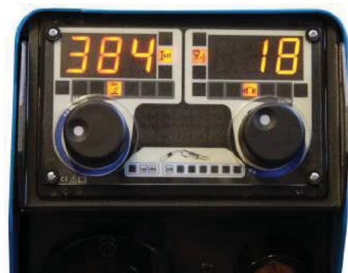
Figure 14. Exemplary method for MIG Synergia Here: welding current 384A, arc length 18, 4-cycle.
