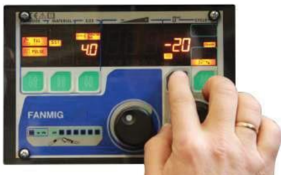
Figure 29. TIG Pulse synergic setting Here: SST stainless steel, tungsten electrode diameter 4.0 mm, -20% pulse correction, 4-cycle with current drop.
