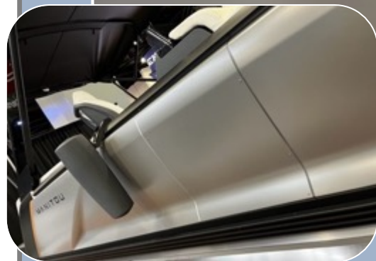
STAMPED & RIVETED PANELS WITH AUTOMOTIVE STYLE "HEADLIGHTS"
