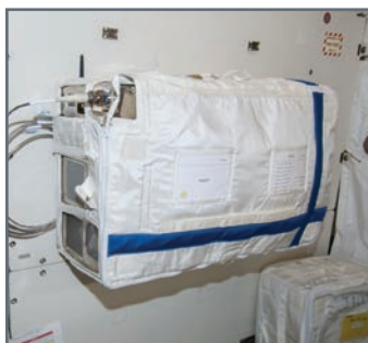
The FROST Installed on JEM1A7-10 panel in the JEM during ISS Expedition 36 (ISS036E037475).
