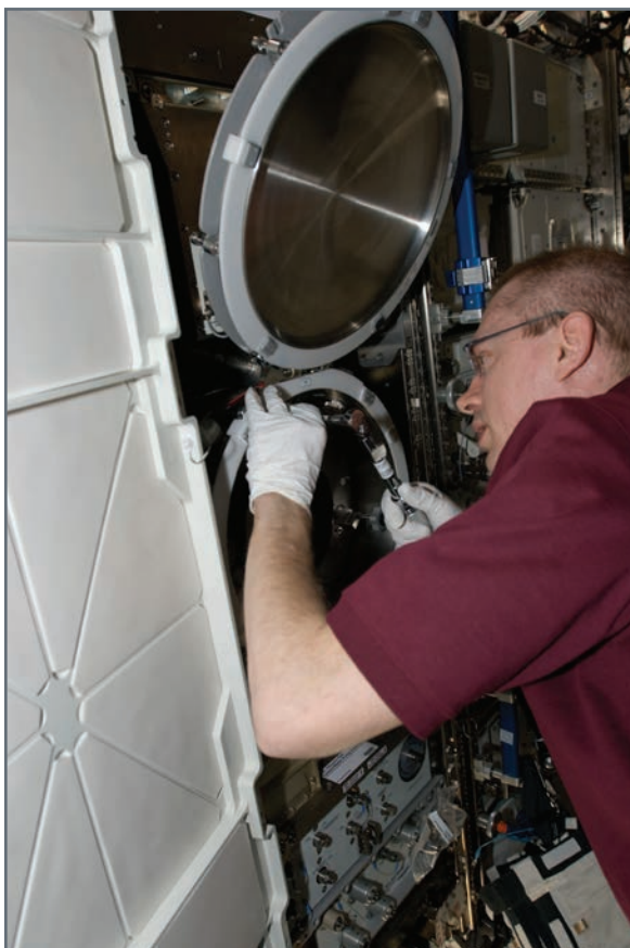
Expedition 21 Commander Frank De Winne reinstalls the MSL Intermediate Support Plate in the MSL Core Facility during MSRR commissioning activities in the U.S. Laboratory/Destiny (ISS021E006227).
