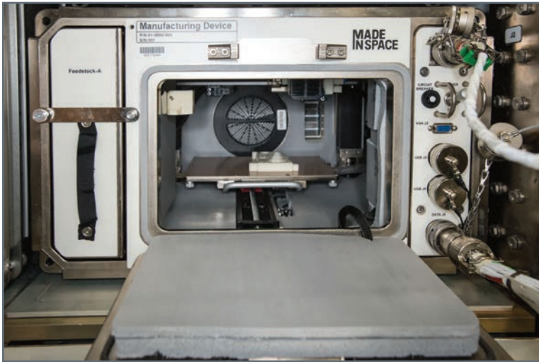
View of the Additive Manufacturing Facility during ISS Expedition 47 print removal (ISS047E152500).
