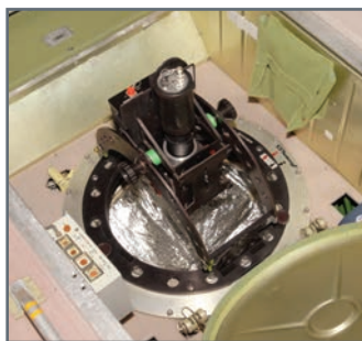
Russian experiment Fialka multispectral ultraviolet system hardware installed on the Service Module/Zvezda window (ISS015E28944).
