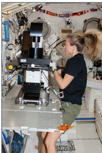
ISS crewmember Karen Nyberg works to set up the JAXA Microscope Observation System (Fluorescence Microscope) in the Kibo laboratory of the ISS during ISS Expedition 36 (ISS036E020972).
