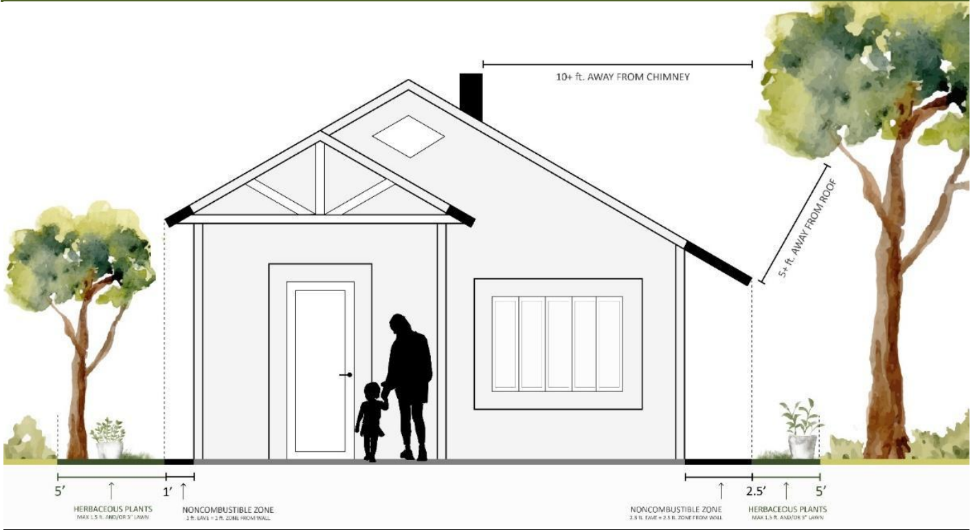
Figure 1: This front view represents how Zone 0 can be divided into a non-combustible “safety zone” immediately near the building, surrounded by a low-combustibility zone out to the remaining 5 feet. A vegetation-free zone would be required at 1 foot from the occupied structure or to the edge of the eaves (whichever is greater); 2 feet from windows, glass doors, and vents; and 5 feet around attached decks, stairs, and pergolas.
