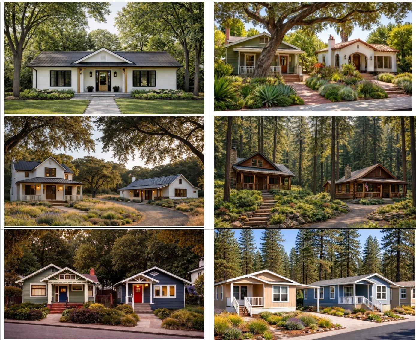
Figure 3. These six homes representing different regions of the state, shown in street view , have been edited in Adobe Photoshop to illustrate how the April 2026 draft of Zone 0 might look in practice over the phase-in period. Note that each house has a non-combustible zone immediately adjacent to the structure, as well as some herbaceous plantings outside the eave dripline. Note that trees are allowed in Zone 0. It is understood that the camera angle affects the perceived impact of Zone 0 on the look and feel of the fire mitigation.
