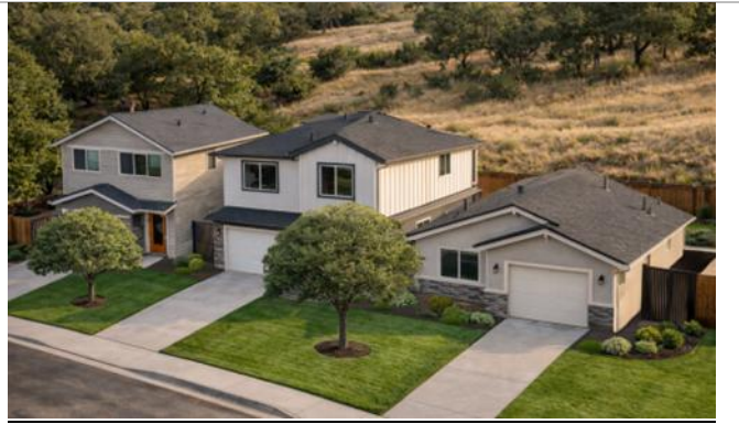
Figure 4. These six example homes, shown in an aerial view , have been edited in Adobe Photoshop to illustrate how the April 2026 draft of Zone 0 might look in practice over the course of the phase-in period. Note that each house has a non-combustible zone immediately adjacent to the structure, as well as some herbaceous plantings outside the eave dripline.
