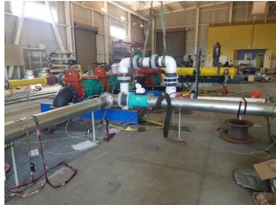
Figure 8 - Technoflos PS 36 flow meter 1-diameter downstream of a simulated pump discharge
