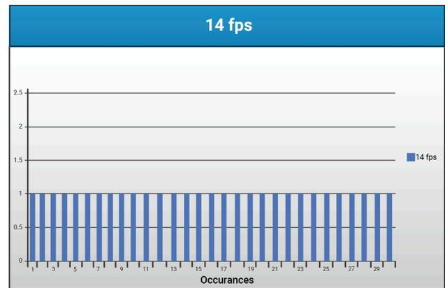
Figure 9 - Histogram of Krohne WF with Pump Upstream illustrating a uniform distribution of errors.
