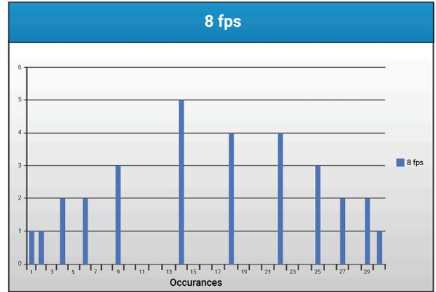
Figure 8 - Histogram of Bermad Euromag 2300 with Pump Upstream illustrating a near bell curve distribution of errors
