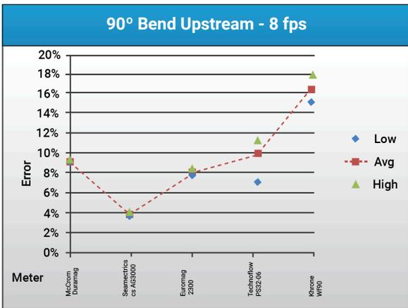
Figure 6 - Graph of the high, average, and low errors as a percent of the average Venturi meter flow rate at 8 fps for the five flow meters.
