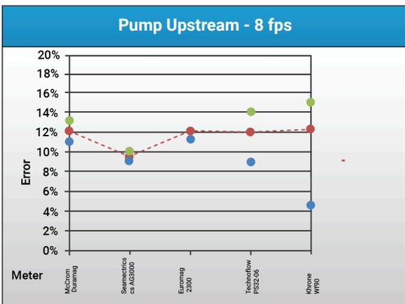
Figure 7 - Graph of the high, average, and low errors as a percent of the average Venturi meter flow rate at 8 fps for the five flow meters.
