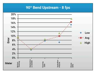
Figure 6 - Graph of the high, average, and low errors as a percent of the average Venturi meter flow rate at 8 fps for the five flow meters.
