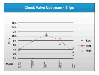
Figure 4- Graph of the high, average, and low errors as a percent of the average Venturi meter flow rate at 8 fps for the five flow meters.
