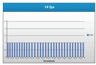
Figure 9 - Histogram of Krohne WF with Pump Upstream illustrating a uniform distribution of errors.
