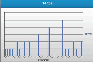
Figure 10 - Histogram of Technoflow PS32 with 90 Bend Upstream illustrating left skew (high number of lower error amounts) of the distribution of errors.
