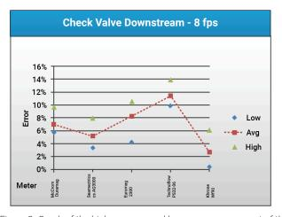
Figure 3- Graph of the high, average, and low errors as a percent of the average Venturi meter flow rate at 8 fps for the five flow meters.
