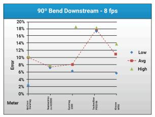
Figure 5- Graph of the high, average, and low errors as a percent of the average Venturi meter flow rate at 8 fps for the five flow meters.
