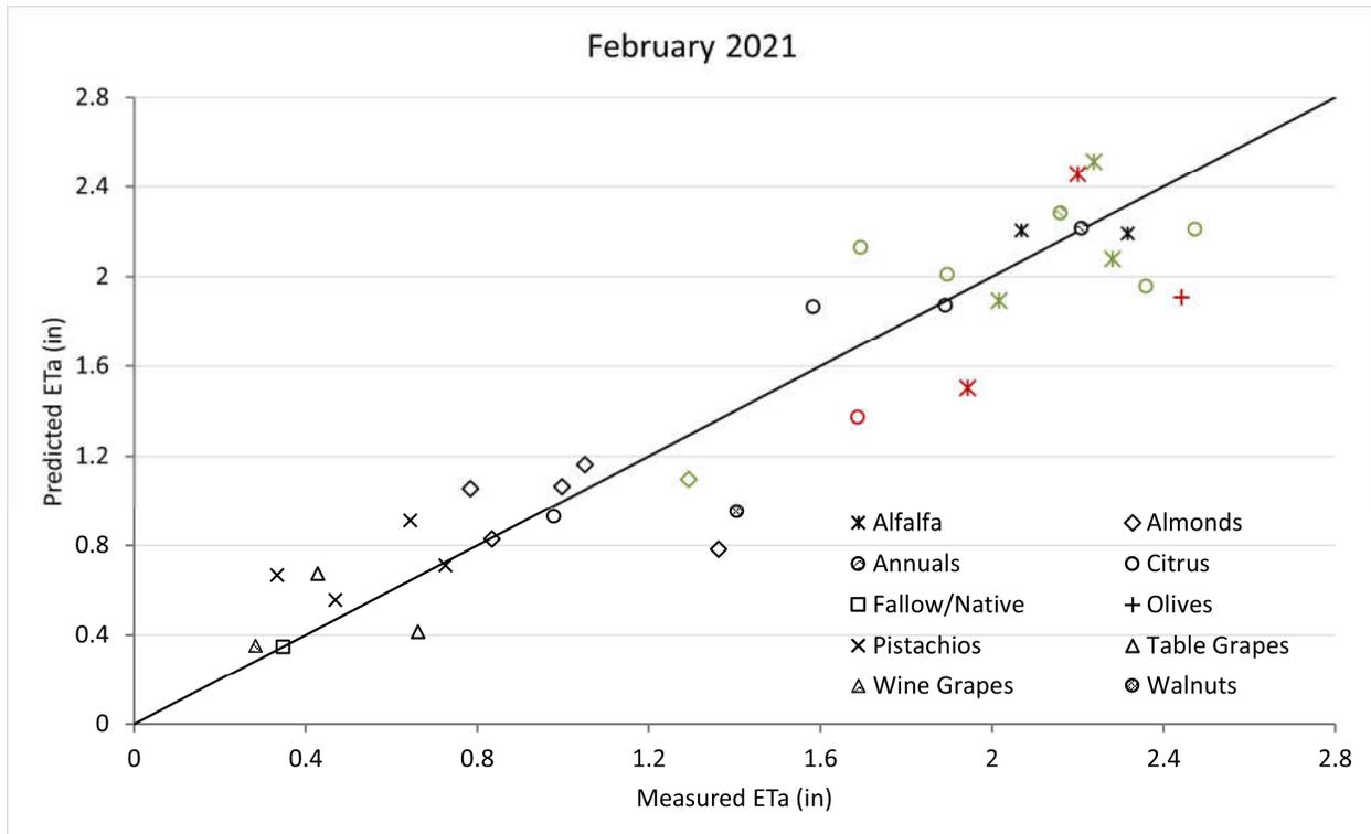
**FIGURE 3. MEASURED VERSUS PREDICTED ET<sub>a</sub> FOR THE MONTH. SYMBOL COLORS REPRESENT THE STATION TYPES (BLACK = FULL, GREEN = WATER IQ (WIQ), RED = TULE TECH)**
