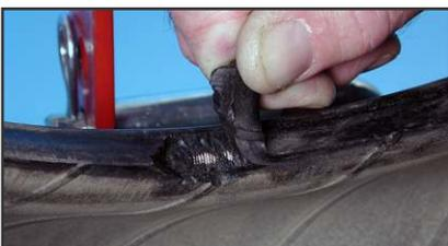
**7.** Deformed bead, exposed fabric or steel
