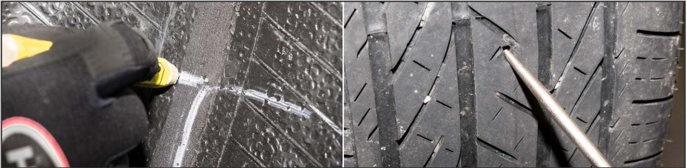
1. Locate and mark all damage on the inside and outside of the tire while checking for separation.
