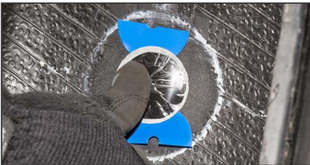
**16.** Press down the repair with your thumb from the center out.
