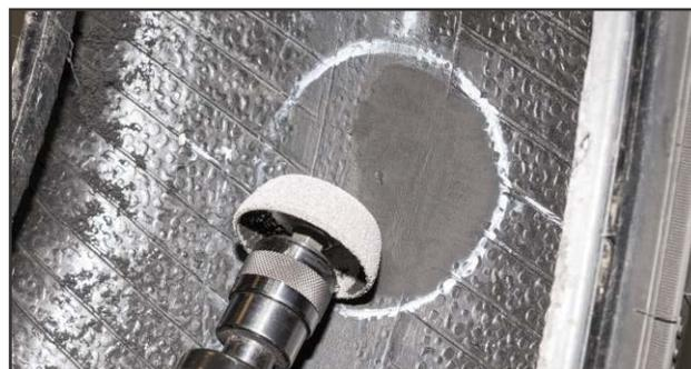
**5.** Using a low speed buffer (maximum 5,000 rpm) and an appropriate inner liner buffing wheel, buff the entire outlined area to a #1 or #2 buffed texture.
