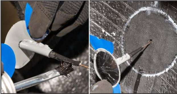
**14.** Apply a small amount of vulcanizing fluid to the black tapered portion of the stem. Relax the beads of the tire. Insert the lead wire through the injury.
