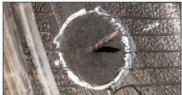
**11.** Allow 3-5 minutes drying time for #760 or 5-8 minutes for #775. Additional drying time may be necessary in adverse weather conditions. Vulcanizing Fluid must be completely dry.
