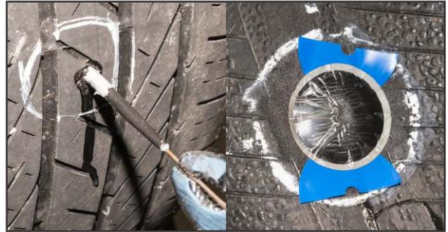
**15.** Grasp the wire with pliers and pull the stem through the tire until the cap forms a slight indentation.
