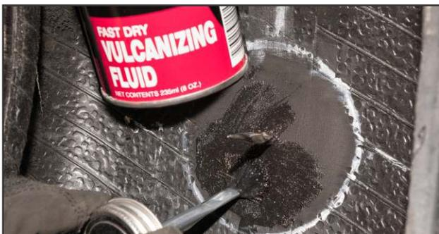
**10.** Apply a thin, even coat of Chemical Vulcanizing Fluid #760 or Heavy Duty Blue Vulcanizing Fluid #775 to the buffed surface.
