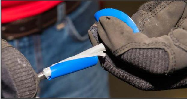
**12.** Remove the blue poly from the stem by pulling and twisting the repair as shown.
