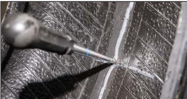
2. Determine the size and angle of the injury using the TRT105 injury measuring tool. If the angle exceeds 35 degrees, a two-piece repair must be used.
