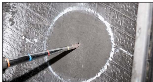
**7.** The injury should be inspected after drilling is complete by flexing the tire and probing the injury with a pointed awl to make sure all splits and loose material have been removed.
