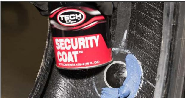
**20.** Seal the edge of the repair and the over buffed area of the inner liner with Tech Security Coat #738 or Butyl Liner Repair Sealer #739.
