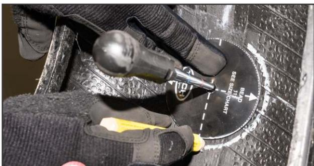
**4.** Outline the area to be buffed 1/2" larger than the repair or use the appropriate repair template.
