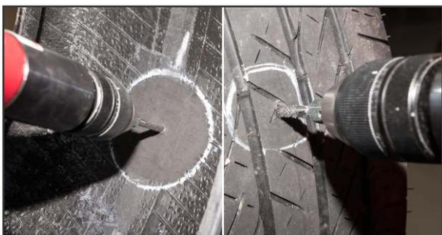
**6.** Damaged rubber and steel should be removed from the injury using a carbide cutter on a low speed air/electric drill, maximum 1,200 rpm. Drill the injury from the inside of the tire 3 to 5 times, followed by 3 to 5 times from the outside. In passenger tires, drilling the injury can be done with a 2,500 rpm air buffer as long as care is taken not to scorch the injury channel.
