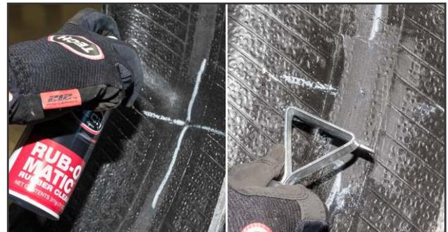
3. Pre-clean the inner liner with Rub-O-Matic Rubber Cleaner #704 or #704A and a scraper 2 to 3 times to remove contaminants.
