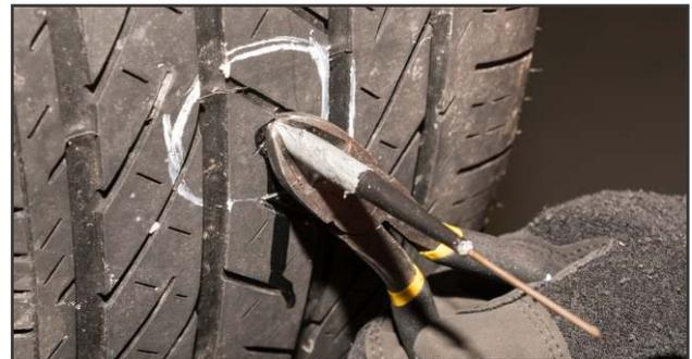
**21.** With the stem relaxed, cut off the excess 1/8" (3mm) above the tread surface.
