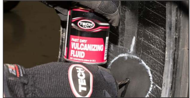
**9.** Using a fluted cement tool for injuries 6mm (1/4") or smaller or a spiral cement tool for larger punctures, apply Chemical Vulcanizing Fluid #760 or Heavy Duty Blue Vulcanizing Fluid #775 to the injury 3 to 5 times.
