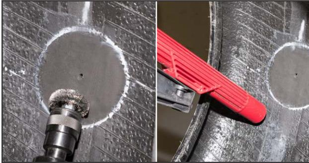
**8.** Use a soft wire brush on a low rpm buffer to remove buffing debris. Do not apply excess pressure as this could alter the buffed texture and reduce repair adhesion. Remove all debris from the tire using a vacuum, being careful not to contact and contaminate the buffed surface.
