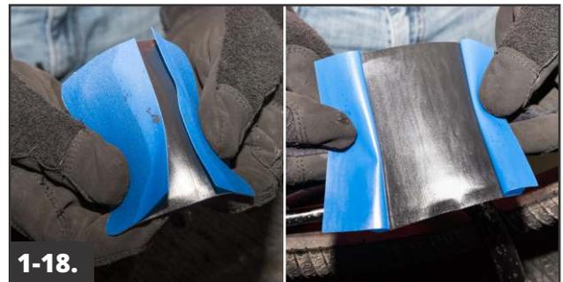
**1-18.** Bend the repair unit back and push up on the edges of the repair with your fingers to break the perforation on the protective poly on the back of the repair. Partially remove the poly, exposing only the middle portion of the repair unit.
