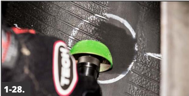
Using a fine grit buffing wheel on a low RPM air buffer (5,000 RPM max), buff the marked area on the inner liner to a #1 or #2 buffed texture, staying within the marked area.
