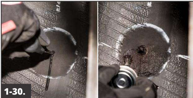
Using a spiral cement tool, apply Chemical Vulcanizing Fluid #760 into the injury 3 to 5 times to ensure the cement is coating the entire injury channel. Leave the cement tool in the injury after the last application. Next, apply a thin, even layer of Chemical Vulcanizing Fluid to the entire buffed surface. Allow 3-5 minutes for Chemical Vulcanizing Fluid to completely dry. Additional drying time will be needed in cold or humid conditions.
