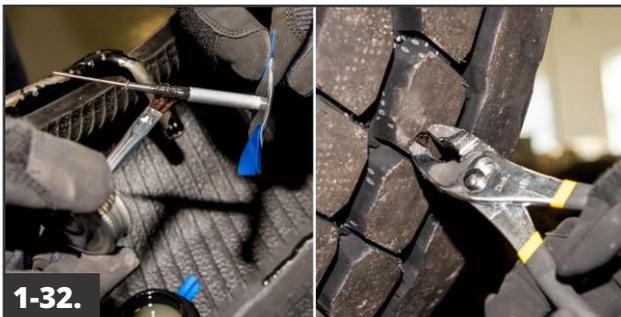
Apply Chemical Vulcanizing Fluid to the tapered part of the stem only and insert the lead wire through the injury from the inside of the tire. Grasp the wire with pliers on the outside and pull the stem through the tire until the cap forms a slight indentation. Do not over pull the stem.
