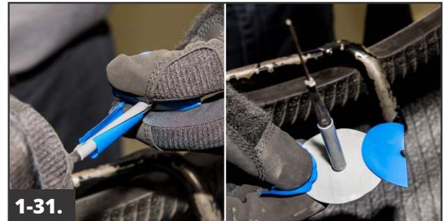
Remove the poly from the stem by pulling on the tapered portion of the stem and twisting until it releases. Remove and reposition the poly on the cap to prevent contamination of the cushion gum and to allow for easier removal of trapped air from under the repair during installation.
