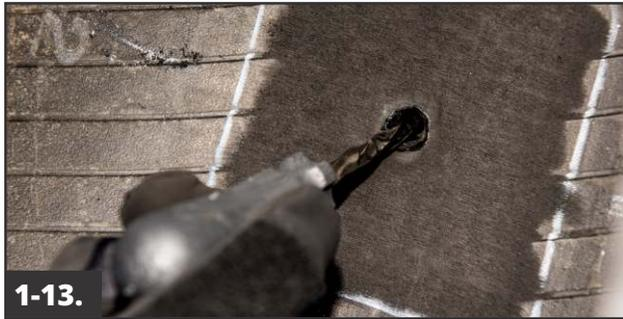
**1-13.** Using a fluted or spiral cement tool, apply black TemVulc cement into the injury.
