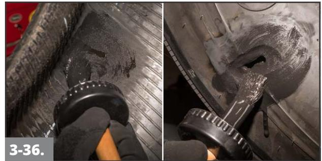
**3-36.** Apply a thin, even coat of Temvulc Black Cement #1082 to the buffed surfaces on both the inner liner and the outside skive. Allow to dry 8-10 minutes. More drying time may be necessary in cold and/or humid conditions.
