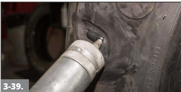
**3-39.** Pre-heat the extruder gun. Exerting firm pressure on the extruder, apply TRRP or LRRP rope rubber into the injury channel from the outside of the tire.
