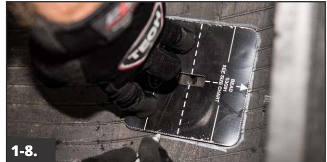
Select the correct repair unit to be installed. Center the proper repair unit template over the injury and use a tire marker to outline the template for buffing. It is also acceptable to use the repair unit and mark an area at least 1/2" (13mm) larger than the repair unit for buffing.
