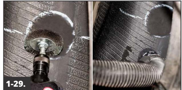
Clean the buffed surface with a soft wire brush on a low RPM air buffer, working from the right side of the buffed area to the left. Repeat until all buffing dust is removed. Vacuum all buffing dust from the tire. Do not touch the buffed surface with the vacuum, as this will lead to contamination.
