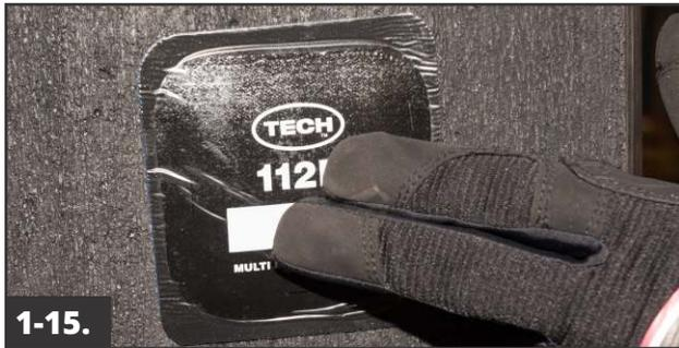
**1-15.** Preheat the extruder. Place a repair unit or a piece of poly over the hole on the outside of the tire. Hold firm pressure against the tire so that no air will be trapped.
