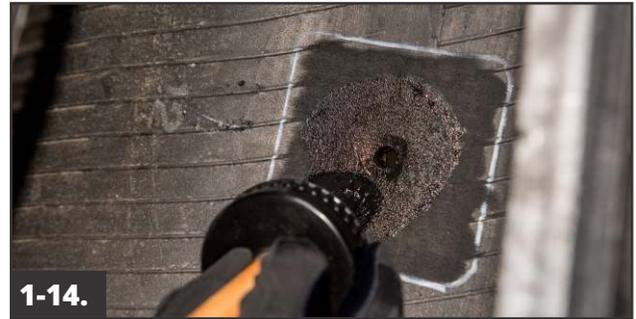
**1-14.** Apply a thin, even coat of TemVulc cement to the buffed surface. Allow the cement to dry for 8-10 minutes. In cold and/or humid conditions, additional drying time will be needed.
