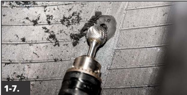
Using a small ball rasp, remove a small area of the inner liner around the injury to inspect the casing. If splits in the rubber and/or loose cables are detected, the damage must be removed. This can be accomplished by using a larger carbide cutter. If the damage is still within puncture limitations, then proceed to the next step. If not, then proceed to the Crown Section Repair procedures on page 10 of this manual.
