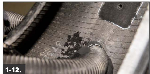
Vacuum all buffing dust from the tire. Do not touch the buffed surface with the vacuum, as this could lead to contamination.
