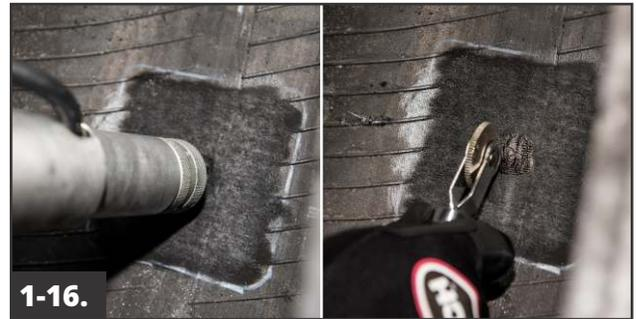
**1-16.** Fill the hole from the inside of the tire with LRRP rope rubber until there is a small amount of rubber above the inner liner. If a non-reinforced repair unit is used, a small amount of overfill is necessary to prevent the appearance of dimpling in the repair unit after curing. Stitch the rubber into place with a stitcher. If too much rubber remains, use a flexible knife to remove the excess rubber to avoid trapping air under the repair unit, then stitch the rubber again.
