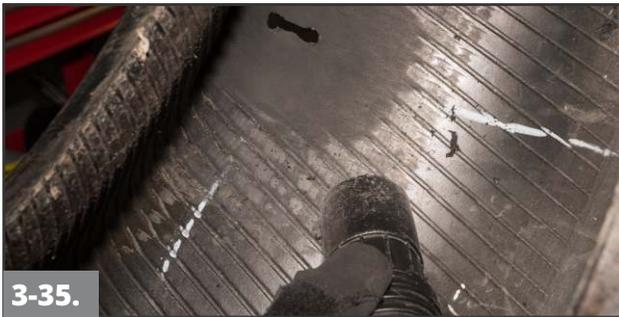
**3-35.** Vacuum all of the buffing dust from the tire. Do not touch the buffed surface with the vacuum as this could lead to contamination.
