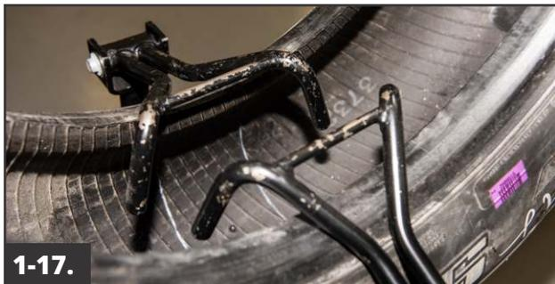
**1-17.** Release the spreader so the tire is in a relaxed position before installation of the repair unit.
