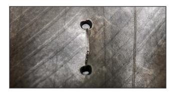
**2.** If the injury is a cut or slit, the ends of the injury must be buttonholed (rounded) in order to prevent injury growth.
