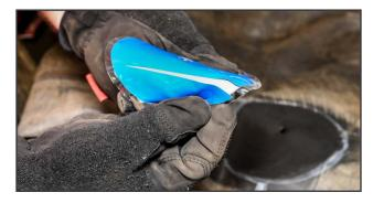
**11.** Fold back the replacement valve and peel back the blue poly backing, exposing the center portion of the cushion gum. Leave the blue cushion gum partially on the repair unit in order to handle the repair without contaminating the gray cushion gum.
