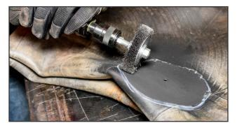
**9.** Use a wire brush or clean lint-free cloth to remove loose debris from the buffed surface.
