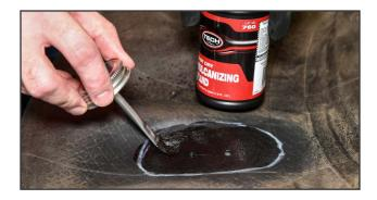
**7.** Apply a thin, even coat of TECH Chemical Vulcanizing Fluid #760 to the entire buffed surface. Allow 3 – 5 minutes to dry. Additional drying time may be necessary in cold and/or humid conditions.
