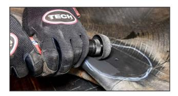
**8.** Using a fine grit buffing wheel or wire brush on a low speed buffer (5,000 RPM Max.), lightly buff the tube to a #1 buffed texture, staying within the marked area. A hand buffer or wire brush may also be used if a pneumatic buffer is unavailable.
