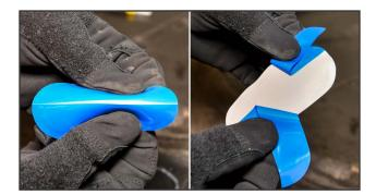
**8.** Fold the repair unit and peel back the blue poly backing to expose the center portion of the repair unit. Leave the blue poly partially on the repair in order to handle the repair unit without contaminating the cushion gum.
