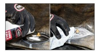
**16.** Apply TECH Tire Talc #706-1 to the replacement valve. This will prevent the gray cushion gum from adhering to the tire. The tube is now ready to be returned to service.
