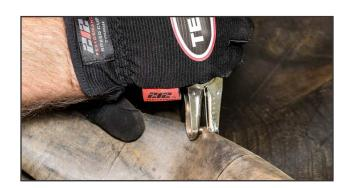
**4.** Move at least ¼ of the way around the tube and punch out a new hole for the replacement valve.
