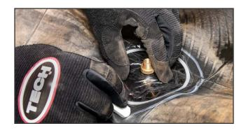
**6.** Mark a perimeter approximately ½" (13mm) larger than the replacement valve as a guide for buffing. If necessary, also draw a guide line on the tube in the same direction as the original valve stem for proper alignment of the stem through the rim opening.
