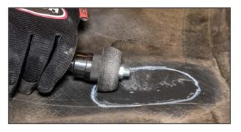
**5.** Using a fine grit buffing wheel or wire brush on a low speed buffer (5,000 RPM Max.), lightly buff the tube to a #1 buffed texture, staying within the marked area. A hand buffer or wire brush may also be used if a pneumatic buffer is unavailable.
