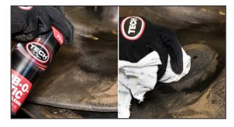
**3.** Pre-clean a large area around the injury using Rub-O-Matic Rubber Cleaner #704 or #704A and a clean, lint-free cloth to remove contaminants. **NOTE:** If the tube is of Natural Rubber construction, DO NOT use Rub-O-Matic, as this could further damage the rubber.
