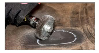
**6.** Use a wire brush or clean lint-free cloth to remove loose debris from the buffed surface.
