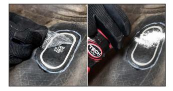
**11.** Remove the clear poly from the top of the repair unit. Apply TECH Tire Talc #706-1 to the repair unit. This will prevent the repair from adhering to the inside of the tire.
