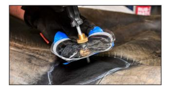
**12.** Use a blunt object to align the valve opening with the hole in the tube. Be sure that the guide lines on the tube and the replacement spud are aligned.
