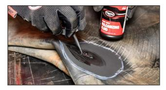
**10.** Apply a thin, even coat of TECH Chemical Vulcanizing Fluid #760 to the entire buffed surface. Allow 3 – 5 minutes to dry. Additional drying time may be necessary in cold and/or humid conditions.
