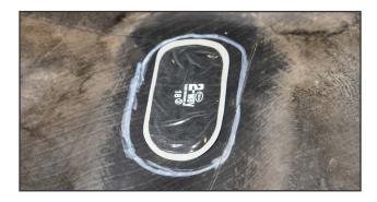
**4.** Select the proper size tube repair for the injury. The repair unit must extend at least  $\frac{1}{2}$ " (13mm) beyond the edge of the injury in all directions. Center the repair unit over the injury. Draw a perimeter, approximately  $\frac{1}{2}$ " (13mm) larger than the repair unit as a guide for buffing.
