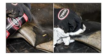
**5.** Pre-clean a large area on the tube using Rub-O-Matic Rubber Cleaner #704 or #704A and a clean, lint-free cloth.
