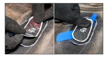
**9.** Center the repair unit over the injury and press it down with your thumb.
