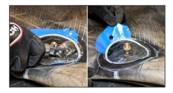
**14.** Stitch thoroughly from the center out. Remove the remaining blue poly and continue stitching out to the edges.
