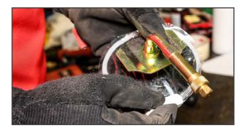
**7.** Tighten the replacement valve stem onto the spud. Now draw a guide line under the valve stem to ensure proper alignment and to guard against air loss.
