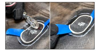
**10.** Stitch the repair unit thoroughly from the center out. Remove the blue poly from under the repair unit and continue stitching from the center out to the edges.
