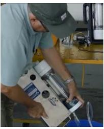
Tipping the unit inverted and pour out the cleaning liquid.
