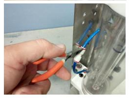
Reinstall Red retainer ring in to the fitting. Run the unit for a minumum of 10 minutes to flush out any residual cleaning liquid. DO NOT consume the water that is purified during the 10 minutes of flushing.
