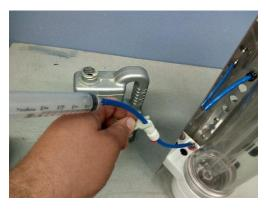
Retract the syinge plunger completely and using the John Guest wrench. Press the locking ring with the wrench and pull the blue syringe tube out of the fitting. Dispose of the used liquid in the syringe.
