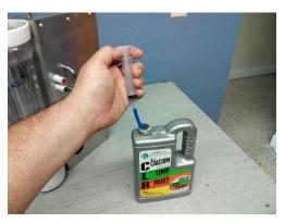
From the tool kit retreve the syringe and the small blut tube. Press the blue tube on to the end of the syringe. Then fill the syringe with CLR or Vinger.
