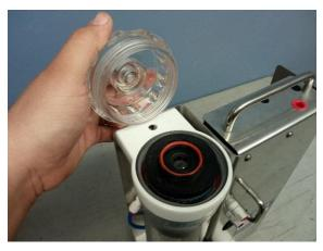
WARNING!!! Removing Ultraviolat Light chamber cap with electrical power ON will expose Ultraviolet Light source. To protect against eye damage, <u>always unplug</u> electical power befor servicing.
