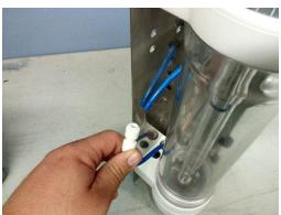
Reinstall the blue tube by pressing the tube securely into the fitting.
