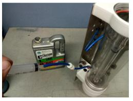
Insert the blue tube in to the fitting on the side of the unit thus connecting the syringe to the unit and squeese the liquid through the blue tube and into the bottom of the UV chamber. Retract the syring plunger effectively pumping the liquid back and forth through the venturi and cleaning it. Continue to pump the liquid for about a minute or until the liquid flows freely.
