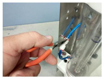
Using Needle nose pliers remove red lock ring from the top of the fitting on the side of the unit. (blue tube)
