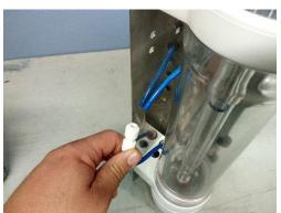
Using the John Guest wrench press down on the top of fitting and pull out the blue tube.
