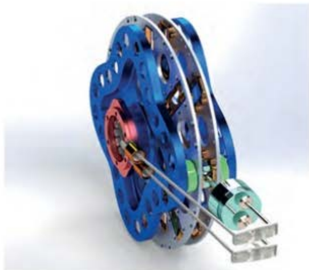
The valve cams (yellow) are bolted around the outer driveshaft, atop the upper driving cam
