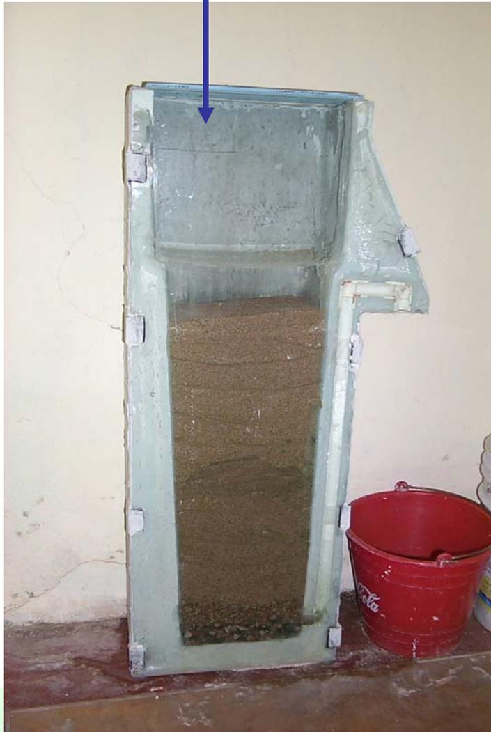
**- Untreated water enters filter when the lid is removed and water is poured in directly.**
