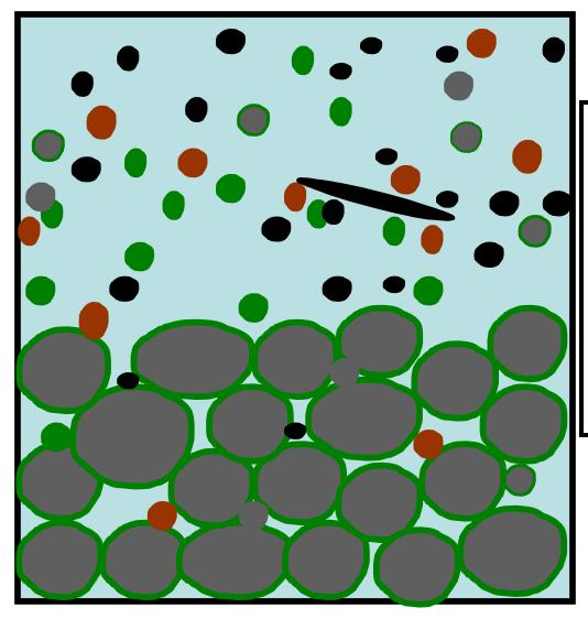
When the agitation is stopped, the media particles coated with a biofilm will settle back into place. The previously captured particles will remain suspended in water above top of media.
