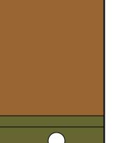
All water is decanted. Note that captured particles cannot penetrate below top layer of media.
