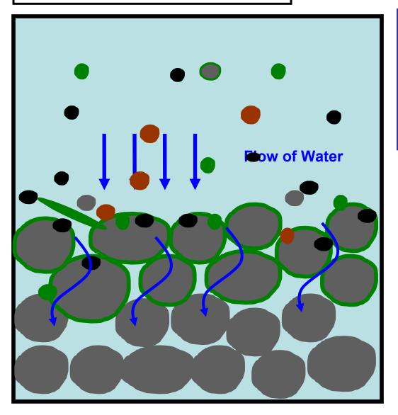
Formation of biolayer will depend on the ecology of the water being treated and the quantity of water being treated. The greater the concentration of aquatic life and the greater the quantity of water being treated the faster the biolayer will form.
