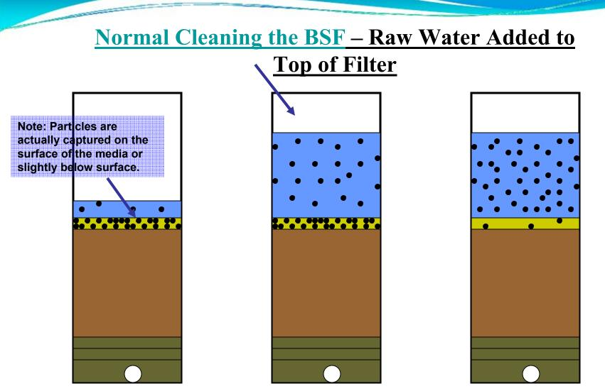
Water level in filter is at the paused depth – could be at any depth.
