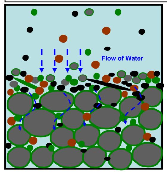
The scraping process will remove the biolayer.
