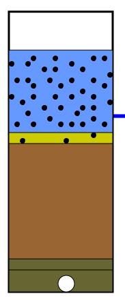
Water containing all of the captured media is decanted from filter surface.
