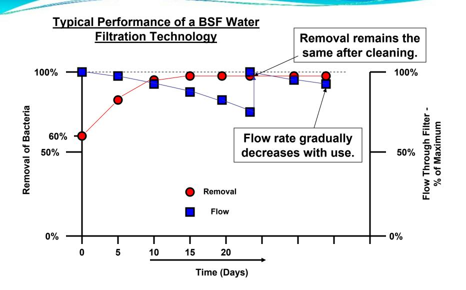
Note: Unlike other water filtration technologies, cleaning of the BSF produces very little waste water. Normal cleaning may be performed with untreated water.
