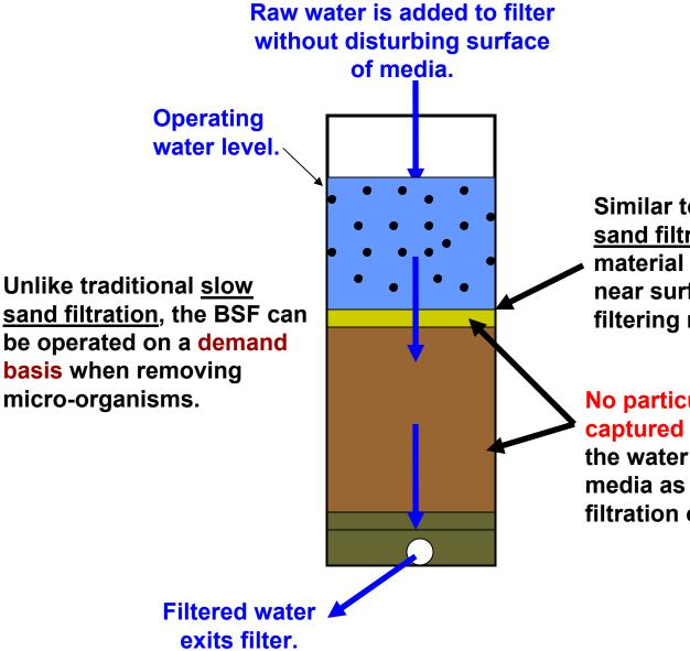
Similar to traditional <u>slow</u> <u>sand filtration</u>, particulate material is captured on or near surface of the very fine filtering media.
