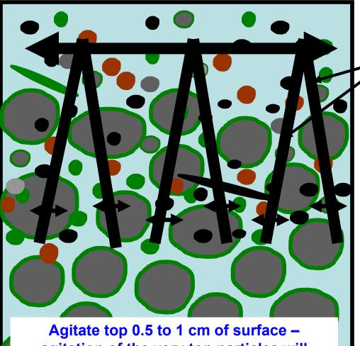
Agitate top 0.5 to 1 cm of surface – agitation of the very top particles will disturb particles below. Wire 'fingers' or real fingers used to agitate <u>very top</u> of filtering media where the particles restricting flow are located.
