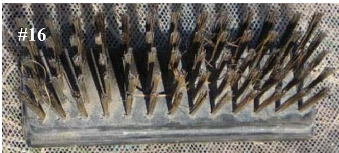
16. Wire brush for cleaning steel mold.
