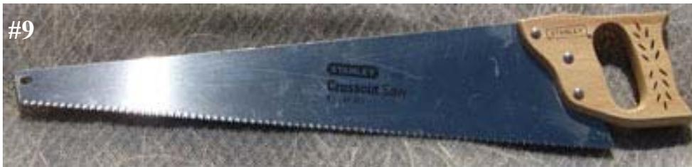
9. Wood cross-cut saw – to fit tool box.
