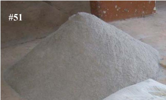
51. Fine crushed rock for use in filter.
