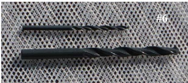
5. Steel drill bits for use in hand drill.
