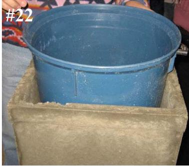
22. Bucket that fits into top of concrete filter and on top of the ledge inside filter.
