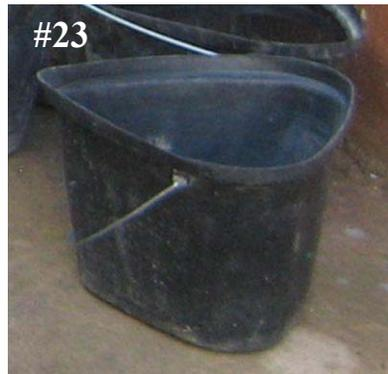
23. Bucket for handling water, sand, gravel and concrete.
