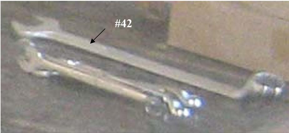
42. Large wrench (spanner) for use with steel mold as shown below.
