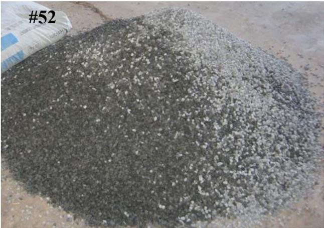
52. 6mm to 12.5 mm crushed rock for use in filter.
