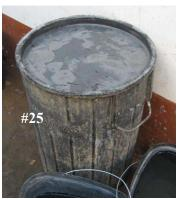
25. Large plastic container for saving water used for washing sand and gravel. Water can be recycled.
