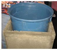
22. Bucket that fits into top of concrete filter and on top of the ledge inside filter.
