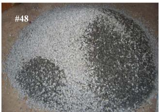
48. Crushed rock for use as gravel aggregate when making concrete.
