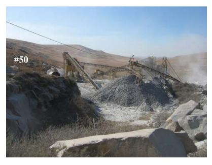
50. Quarry for crushed rock used for filter media.
