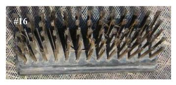
16. Wire brush for cleaning steel mold.
