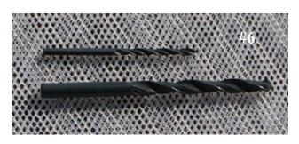
5. Steel drill bits for use in hand drill.3 mm (3/8 inch) purchase several as these break.6 mm (1/4 inch)
