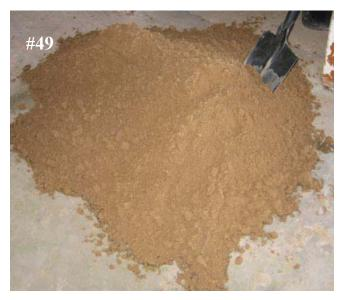
49. Clean construction sand for use when making concrete. May need to be screened to remove large particles, clay and organic material before use.
