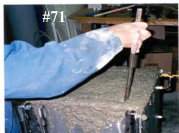
72. Concrete is 'heaped' on top.
