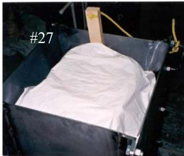
29. Located and ready for leveling. (Make sure there is enough space to allow demolding.)
