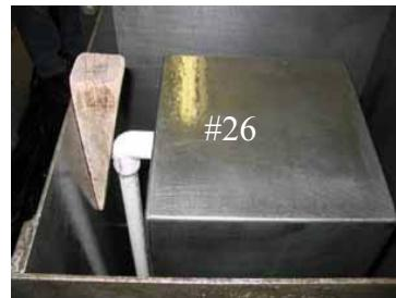
27. Use piece of plastic or paper to cover top of interior mold. This will avoid having the oil removed from surface.
