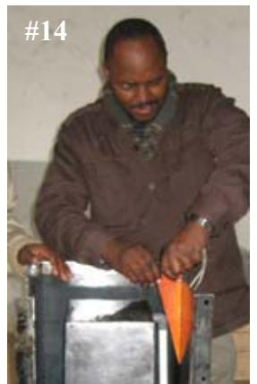
13. Nose piece should fit through 'nose' and exactly between front panel and interior mold. Shorten as required.
