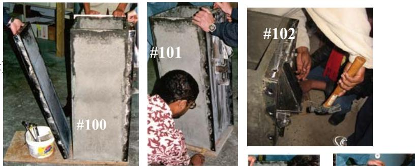
102. Sharply strike the edges of the steel mold with a steel hammer, Gently pull panel out from bottom and up to remove.
