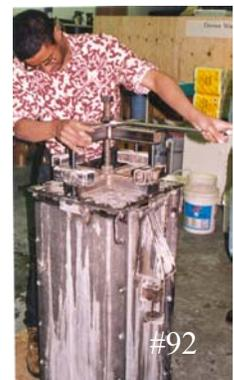
92. Start tightening the puller nut.
