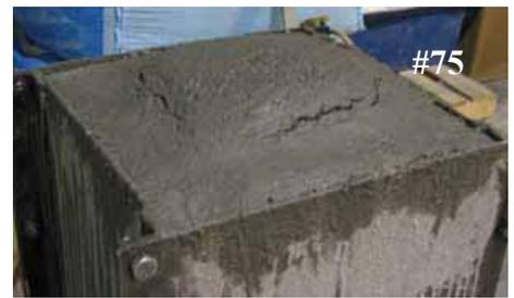
76. Wood wedge is removed. Surface is 'chopped' up using a trowel
