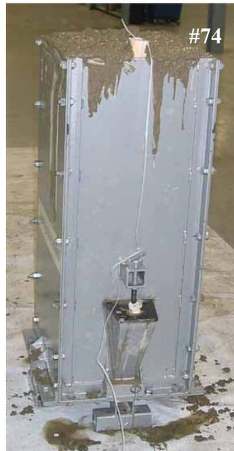
74. Concrete, with wood wedge in place is allowed to 'set' for 3 to 4 hours.
