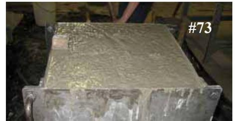
75. After 'setting' and settling cracks will be observed. This is what is expected. Surface is ready for leveling.
