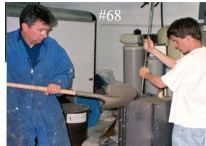
69. **Rodding** the concrete using a steel rod. (Insures that concrete is in all places. Be careful not to disturb standpipe.)
