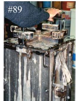
89. Placing puller into holes.
