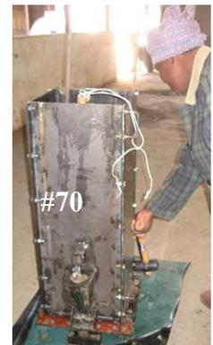
70. Using a rubber hammer to remove air bubbles.
