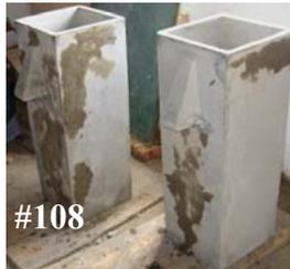
109 – 110. Cleaning and oiling all pieces of the steel mold.
