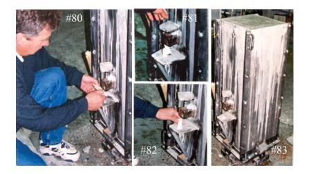
84 – 87. <u>Carefully</u> turning mold unto its base.
