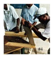
Cutting the boards using the hand saw (not the hack-saw.
