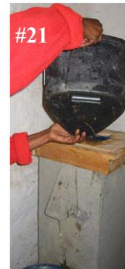
21. Pouring water into filter to start flushing process.
