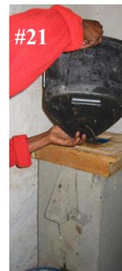
21. Pouring water into filter to start flushing process.
