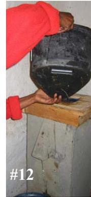
12. Adding more water to filter with diffuser basin in place.
