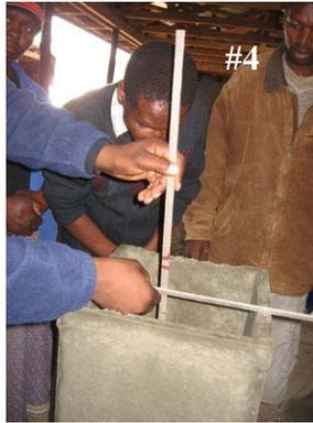
**If thickness of layer is too great some media will be removed. Similarly, if the thickness is too small media is removed. Measurements are taken after the surface of the media is leveled.**
