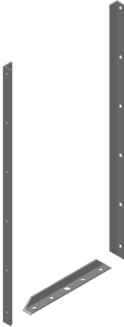
Figure 19a Assembling the front panel - attaching angle iron.
