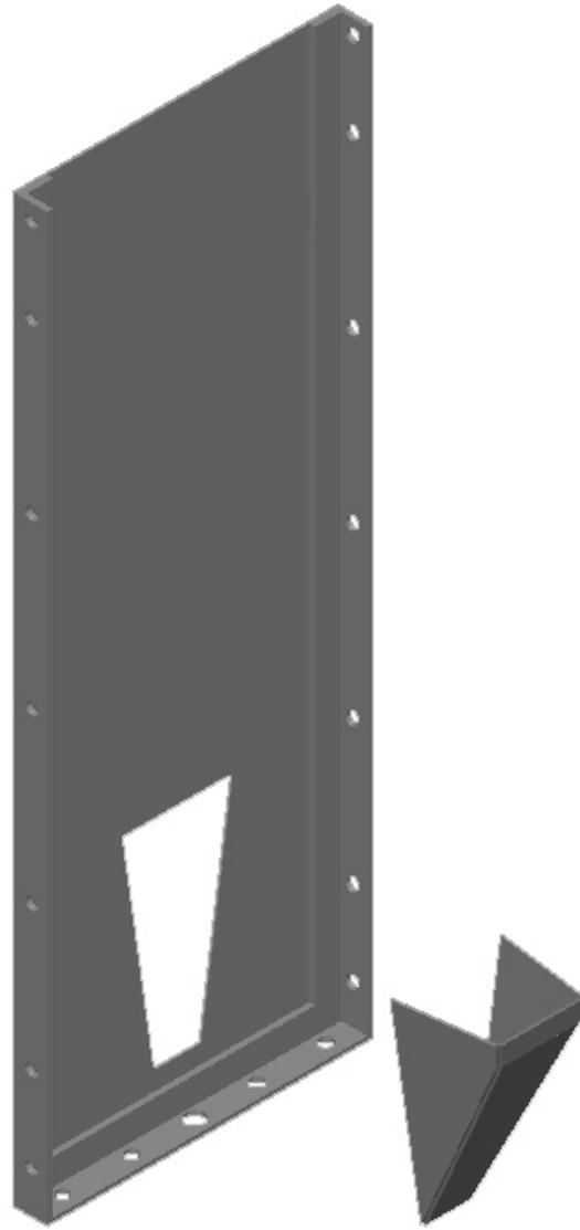
Figure 13a Attaching nose to front panel.
