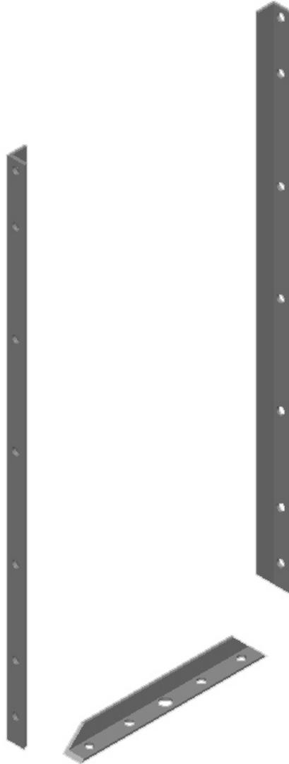
Figure 11a Assembling the front panel - attaching angle iron.
