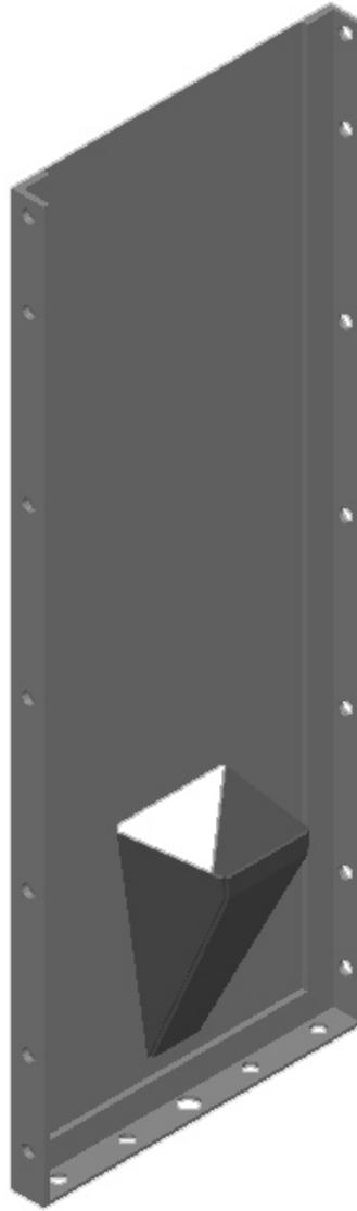
Figure 13d Front of front panel with nose piece attached.
