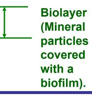
Formation of biofilm on the mineral particles is exactly the same as that observed in 'trickling filters' used for aerobic treatment of wastewater. <sup>5</sup>
