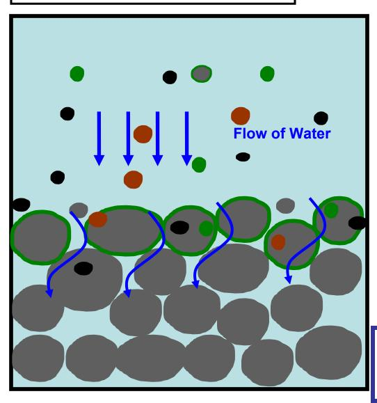
No biolayer is necessary for removal of parasites and larger organic material and mineral particles including oxidized iron and manganese.
