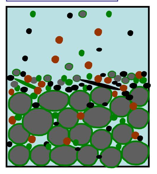
If the water in the filter has been lowered to the paused depth (5 cm) additional untreated water should be added from the top through the diffuser.
