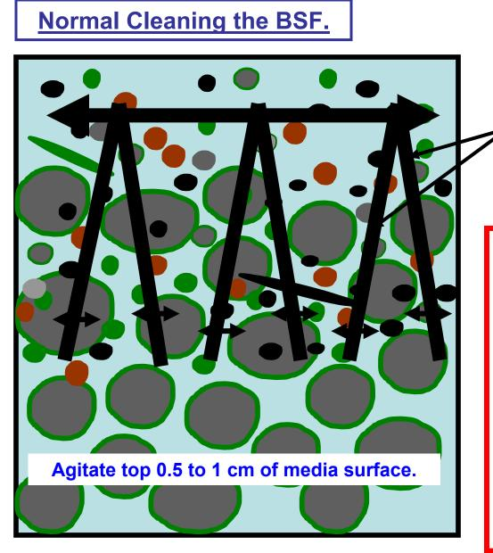
Wire 'fingers', real fingers or a spoon can be used to agitate <u>very top</u> of filtering media where the particles restricting flow are located.
