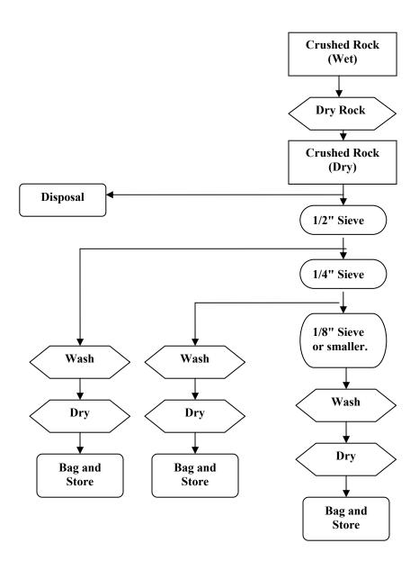
Figure 2. Media preparation flow chart when one crushed rock supply is used to produce media used in the three layer system.
