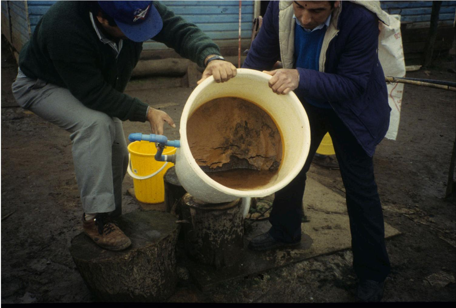
**Iron removal using the BSF in Chile and the discovery of the commercial potential of the technology in Canada.**
