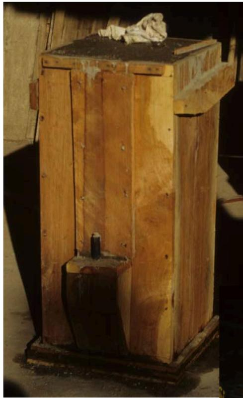
**First concrete filters manufactured using a wood mold.**
