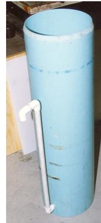
**First prototype of the modern BioSand Filter**
