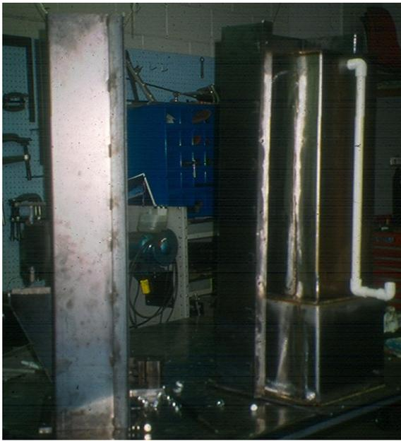
**Development of the first steel mold for construction of the concrete BWF at the University of Calgary.**
