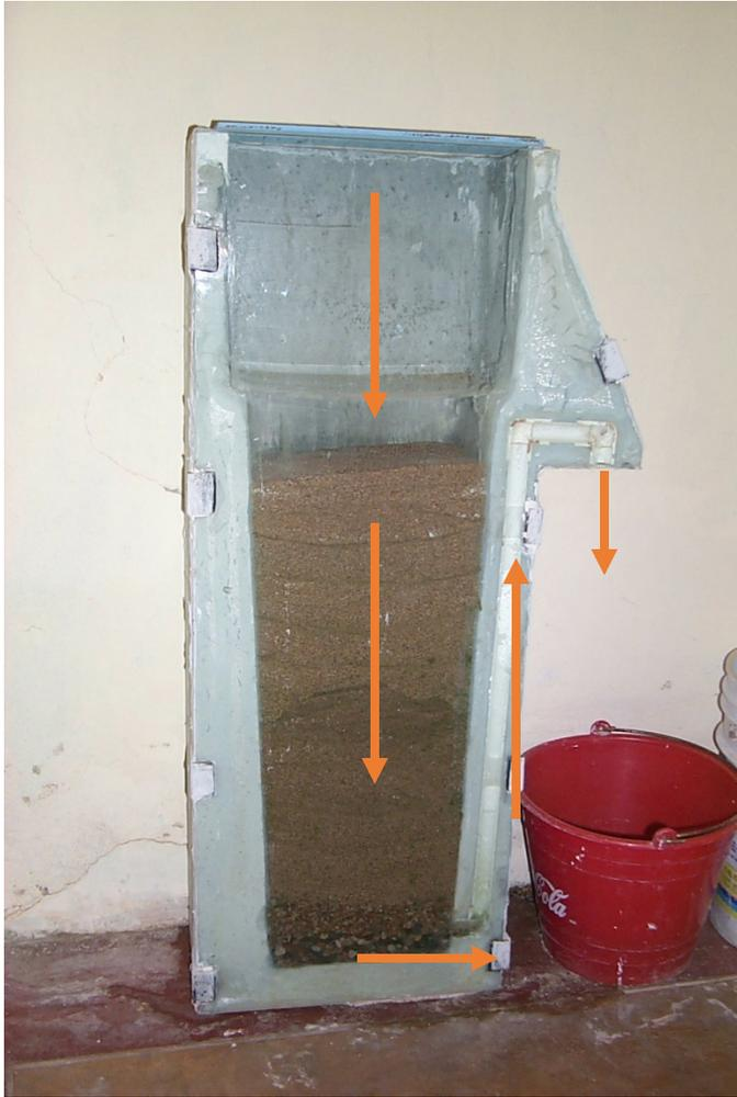
**- Water passes through the sand to the underdrain, up the standpipe and out into the bucket below.**
