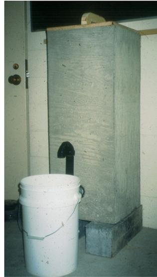
**First cast concrete BSF at U of C.**
