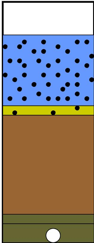
Water containing all of the captured material is decanted from filter surface.
