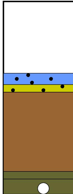
All water is decanted. Note that captured particles cannot penetrate below top layer of media.
