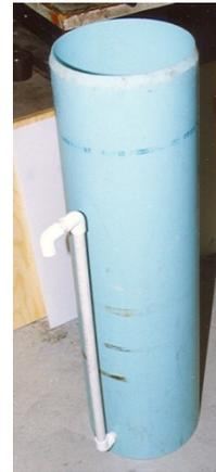
**First prototype of the modern BioSand Filter**
