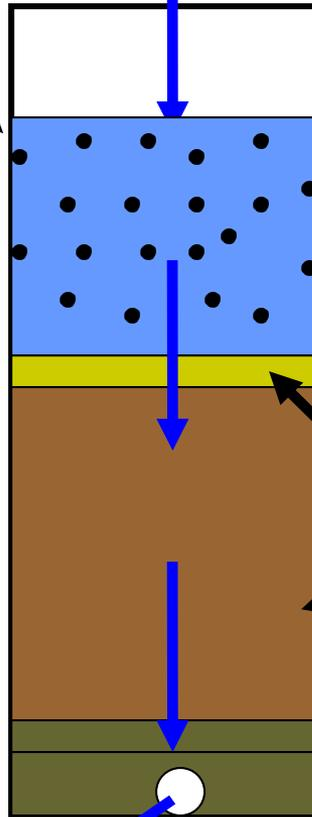
Similar to traditional slow sand filtration, particulate material is captured on or near surface of the very fine filtering media.
