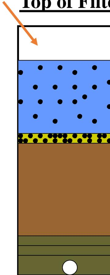
Untreated water is added until there is at least 0.2 to 0.3 m of depth above top layer of media.
