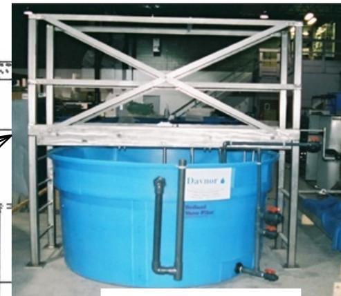
**2,000 lph BioSand Water Filter**
