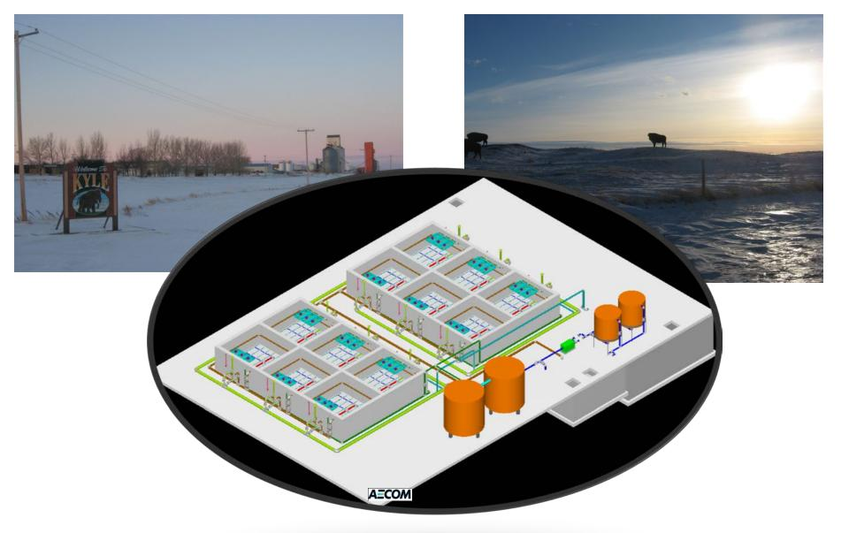
Water treatment plant to remove complexed iron and manganese from groundwater -Saskatchewan, Canada construction completed 2014-100,000 LPH with 100% recycle of wastewater.
