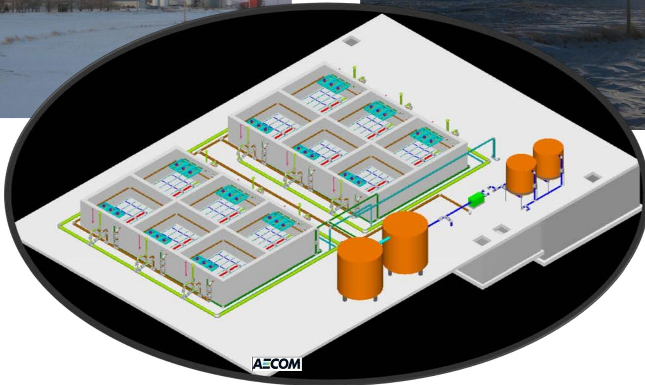
**Water treatment plant to remove complexed iron and manganese from groundwater - Saskatchewan, Canada construction completed 2014- 100,000 LPH with 100% recycle of wastewater.**
