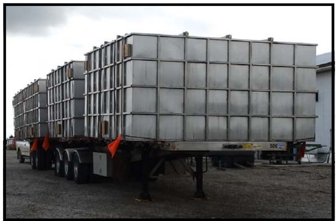
MEL Filter - 4m x 4m x 2m stainless steel body.
