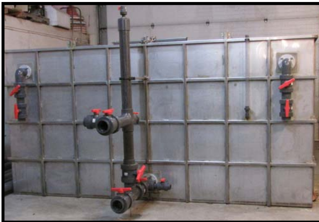
MEL Filter - 4m x 4m x 2m stainless steel body.
