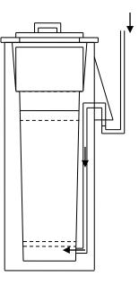
Figure 7. Household concrete BSF with disinfection U-tube attached to outlet of standpipe.
