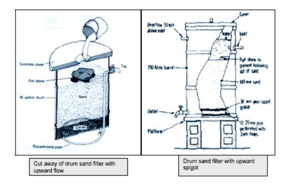
Figure 1. Sand-in-a-barrel filters.
