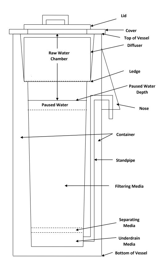
Figure 3. Cross-section of concrete household BioSand Water Filter.
