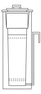
Figure 4. Cross-section of concrete household BSF with plastic standpipe incorrectly installed outside of filter body.
