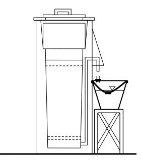
Figure 6. Concrete household BSF producing water into a bucket.
