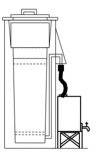
Figure 9. Concrete household BSF with dispensing container and flexible hose connecting standpipe to inside container.
