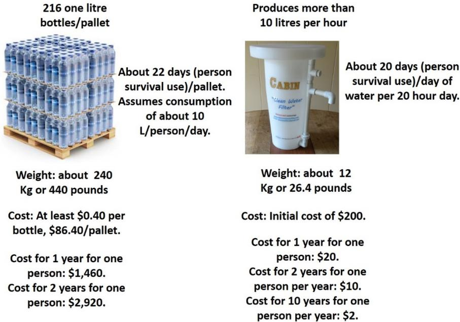
Figure 1. Comparison of the CCWF to supplies of bottled water.
